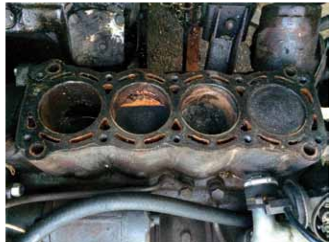
▶ Rost und Dreck in allen Zylindern Rust and dirt in all cylinders
